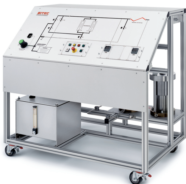
Autofrettage unit for 7,000 bar with two redundant pressure intensifiers for unrestricted availability (Germany). Process sequence is given by a logic controller. Autofrettage pressure is digitally indicated.
