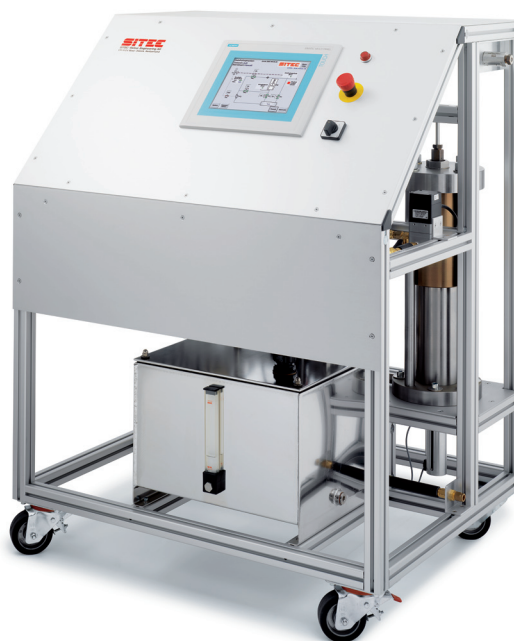
Autofrettage unit for 10,000 bar with PLC process control and batch documentation. Process is visualized on an interactive touch screen. During the autofrettage cycle the pressure curve is indicated and all relevant data are stored in an unchangeable format.
